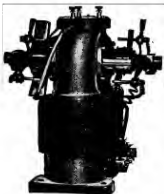
FIGS. 168-169.—Motor-generator central battery ringing machines, the first designed to work from street power circuit; the second, from storage battery at the exchange, both generating an alternating current. The machines are of the type supplied with the exchange battery plants of the Western Telephone Construction Co. The armatures are double wound, the commutator side being the motor, the collector ring side, the dynamo, the same field serving for both.
